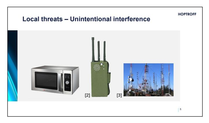
[CLICK] Examples of unintentional interference include [CLICK] microwave ovens, [CLICK] truck drivers using signal jammers to cover their tracks and [CLICK] faulty active antennas in antenna farms that start transmitting rather than receiving
